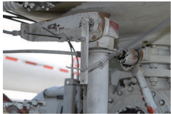
TO OBTAIN FULL OPERATING LEVER TRAVEL WITH SOME CABLE CONTROLS, THE CABLE HAS TO BE ATTACHED CLOSE TO THE HANDLE PIVOT
